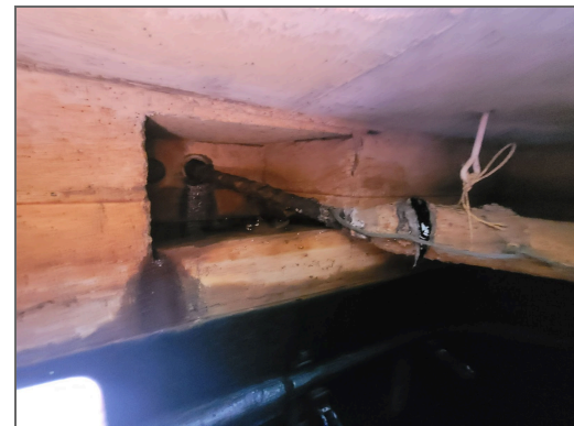
(b) Underground cable failure
